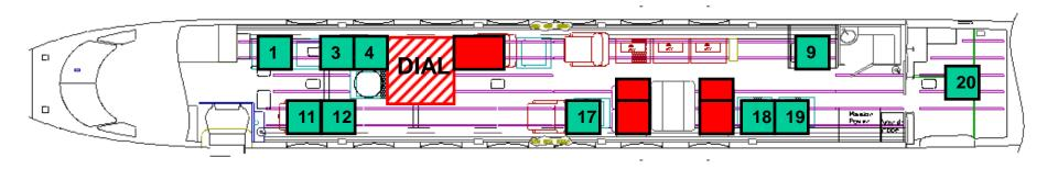
Rack #5, 6, 14, 15 DIAL: Water vapour profiles, aerosol extinction profiles
