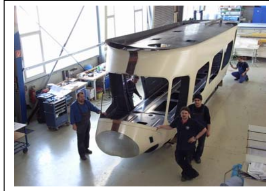
ZEPELIN LZ N07 : Passagiergondel #4 Airship passenger gondola (CFRP)
