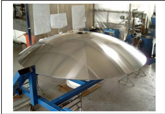
IGN Radioteleskop Subreflektor (HM-CFK) Radiotelescope subreflector (CFRP)
