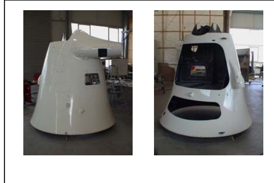
ZEPELIN LZ N07 : Heckantriebsgondel Airship rear engine nacelle (CFRP)
