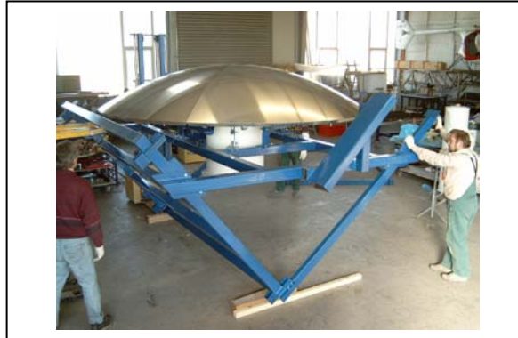
IGN Radioteleskop Subreflektor (HM-CFK) Radiotelescope subreflector (CFRP)
