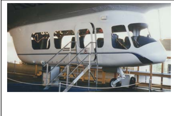
ZEPELIN LZN07: CFK-Passagiergondel #1 Airship passenger gondola (CFRP)
