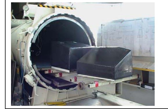
BOEING NET JET :CFK-Trinkwassertanks Potable water tanks (CFRP)
